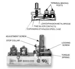
heated surface, a temperature change is sensed almost instantaneously. With an incrase in temperature, the case expands. This results in a linear change of the internal bridge assembly causing the electrical contacts to open. A decrease in temperature closes the contacts.
