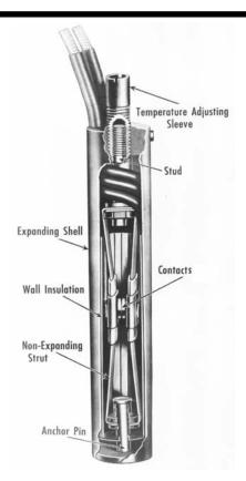
'to "lead" the struts by an interval that varies with the rate of temperature change. With rapid temperature rise, the shell exerts a larger net force on the struts and tends to pull them apart sooner than if the temperature were rising slowly. The result is several degrees or more of anticipation which helps produce closer control.
